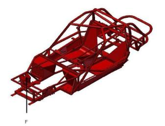
Diagram of chassis showing the position at which ride height measurements will be taken, front (F) and rear (R).
