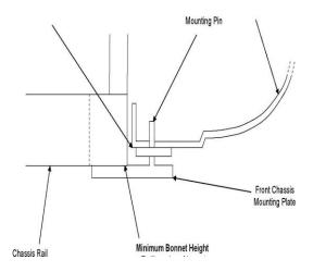
Trailing edge of bonnet can be mounted no lower than the front chassis cross member.
